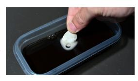
no reaction, the solution is expended. This test should be performed near the end of the recommended circulating time. If near the end of the recommended cleaning time the solution has been expended, more **RYDLYME** will be required to complete the job. However, if the solution is still active at the end of the recommended time, all the scale has been dissolved within the application and it is ready to be water flushed and returned to service.
