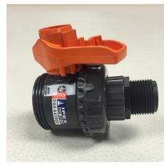
Remove turn valve handle from the top of the true-union ball valve with pre-installed hex nipple. Flip handle over and remove inner Apex Engineering Products cover by pushing through with a pencil or long, thin object.
