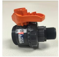
Remove turn valve handle from the top of the tru-union ball valve with pre-installed hex nipple. Flip handle over and remove inner Apex Engineering Products cover by pushing through with a pencil or long, thin object.
