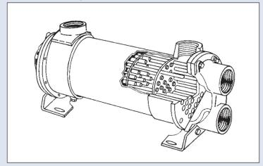
Any type of water cooled heat exchanger can usually be cleaned with *RYDLYME*. Hydraulic oil coolers that become fouled with water scale, lime and rust deposits will eventually cause a shutdown of expensive production equipment.
