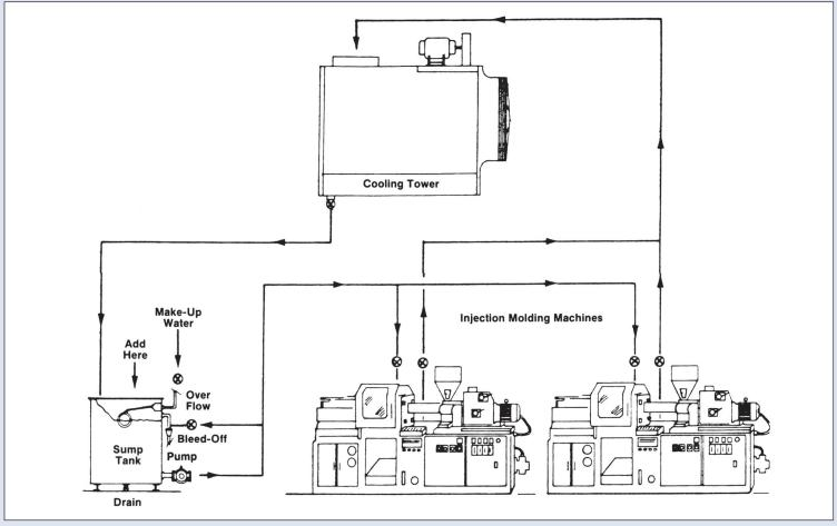
Cleaning of closed circuit water cooling systems is most usually accomplished while the water cooled equipment is on line and without the necessity of a shutdown.
